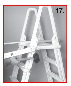
Position the tread connector as shown, with the padlock hole facing upward, and tap it over the round knob. Repeat for the opposite tread connector.
