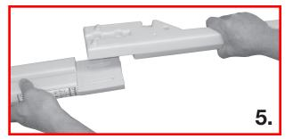
Place handrail over the flat area located on top of ladder leg. Insert one of the 1/4 - 20 x 1" bolts through the ladder leg into the handrail. Place one 1/4 - 20 hex nut into the recessed area on the handrail and tighten using a Phillips screwdriver. Install the second bolt and nut. Repeat to assemble all four ladder leg/handrail assemblies.
