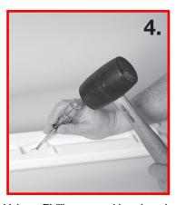
Using a Phillips screwdriver, knock out all four of the keyhole slot inserts from two of the ladder legs.
