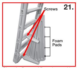
Place the Base and Brace into position, centered, on the bottom and third treads of the ladder. Install the four (4) #10 x 1-1/4" screws (included in hardware pack) on a slight angle, first in the Upper brace, then in the Lower Base. Install the self-adhering foam strips to the Large Barrier Section as shown in diagram.
