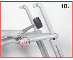
Making sure that the "swing-up" side of the platform is facing away from the "inside" ladder section, as shown, slip the openings of the platform over the upper ends of the ladder legs. Using a mallet or hammer tap the platform With the ladder standing up, tap the down until it is fully seated onto the "nubs" of treads all the way down until seated the ladder legs. Liquid soap or lubricant will help the parts slide together.
