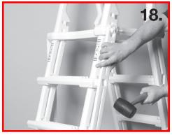
Lay ladder on its side, put a little liquid soap onto the square ends of the treads. Next place the tread connector onto the ends of the treads and strike hard with a rubber mallet to seat tread connector onto the treads. Flip ladder over and repeat for second tread connector.
