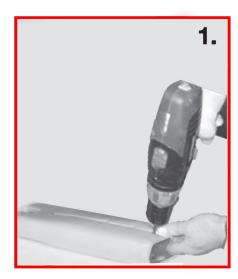
If the round plastic inserts on the sides of the extension boots are still in place, remove them using a drill and a 5/16"s drill bit.
