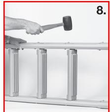
Tap the ladder leg down onto the ends of the treads.
