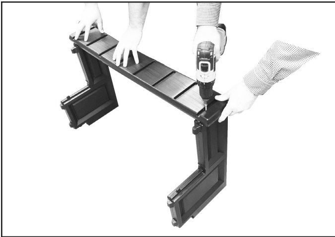
#3: With a helper, place the 5" support over the two locking tabs on the sidewalls. Tap down with mallet until seated on the locking tabs. Secure the support at both ends using 2 - #10 x 1-1/4" screws.
