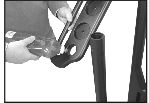
Step 6: Spread dish soap on the openings on the towel bar. This will allow the towel bar to slide over the handrail posts easier.
