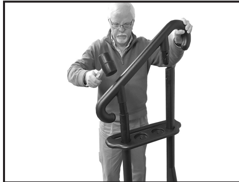
Step 8: Tap the handrails into the handrail posts.
