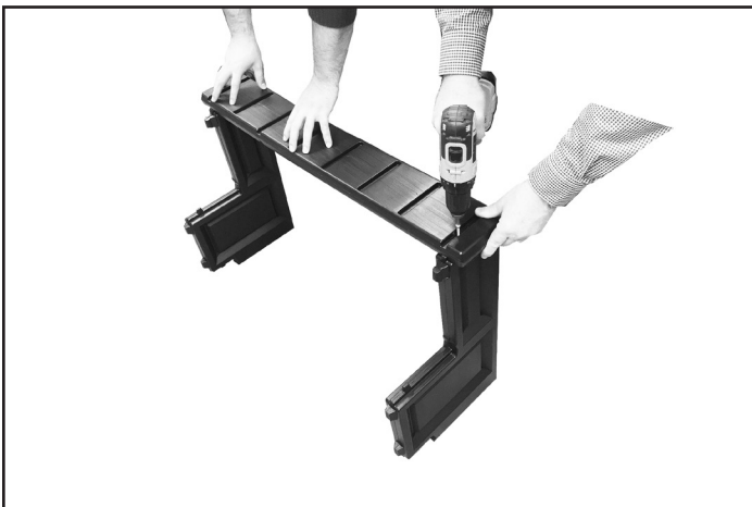
#3: With a helper, place the 5" support over the two locking tabs on the sidewalls. Tap down with mallet until seated on the locking tabs. Secure the support at both ends using 2 - #10 x 1-1/4" screws.
