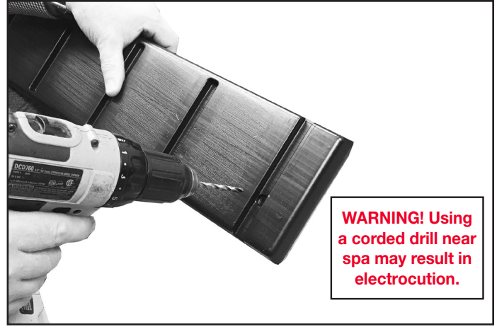
#2: Pre-drill 1/8" pilot holes in the two marked locations at the ends of the 5" support.
