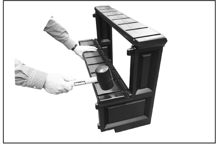
#4: Place the 7" support over the two locking tabs with the groove facing up. Tap down with a rubber mallet until seated on the locking tabs. No screws are required.
