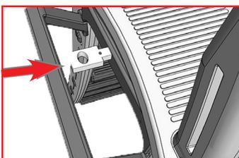
**To close ladder:** Pull down ROLLGUARD® to cover outside ladder treads. To lock, push in the roll guard locking tab located on the left bridge. When properly locked, the ROLLGUARD® will not lift up. Install the padlock through the locking tab hole.
