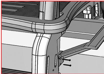
**WARNING!** To stabilize your pool ladder, stabilizer rails must be installed properly and rest on and be attached to the pool top ledge.
