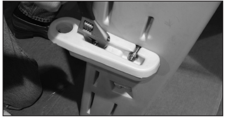
Slide the bottom hinge bracket up on to the bolts and tighten securely.
