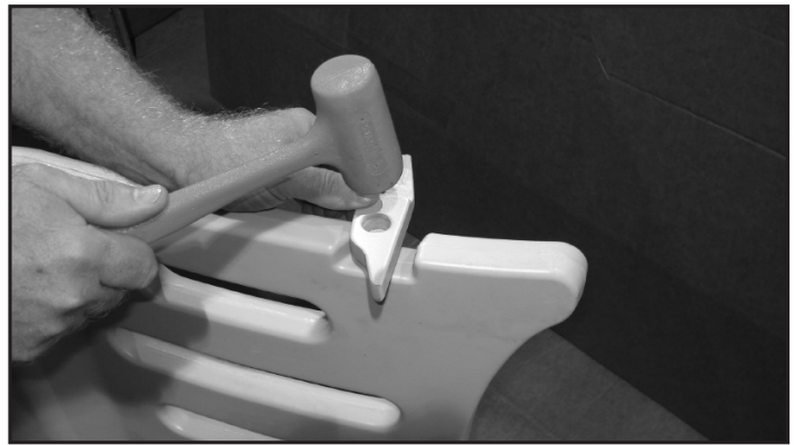
Place the gate on edge and carefully install latch using a rubber mallet. It may require several hits with rubber mallet.
