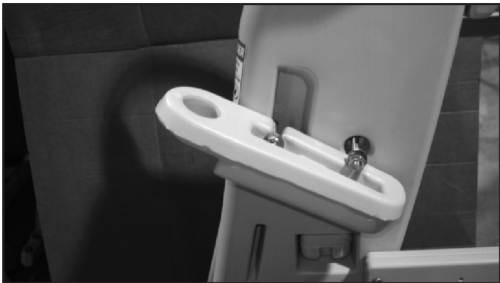
Slide the top hinge bracket on to the bolts as shown and tighten only enough to hold in place.
