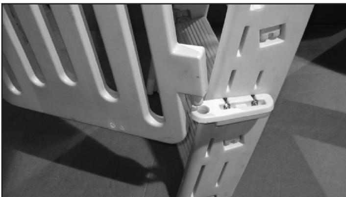
Place the lower gate hinge post in to the lower hinge bracket. Rotate the top hinge bracket up and over the top gate hinge post and tighten bolts.
